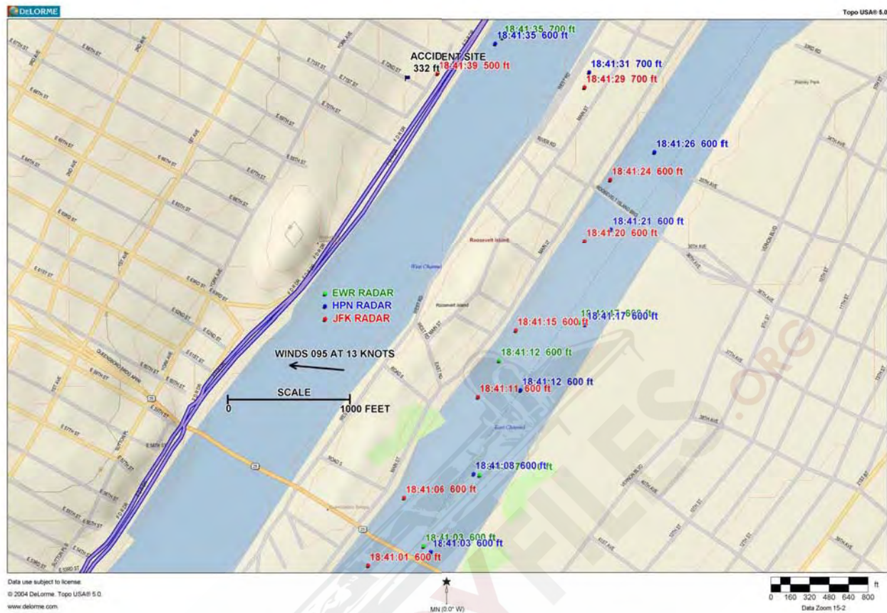
Figure 4. Radar tracks of the accident flight over the East River.
